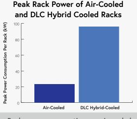
Peak power consumption per air-cooled rack and DLC hybrid-cooled rack.
