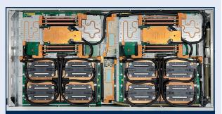
CoolIT's Passive Coldplate Loop (PCL) that provides 100% heat capture on the HPE Cray EX server found in Frontier, <u>the</u> <u>fastest supercomputer in history</u>.
